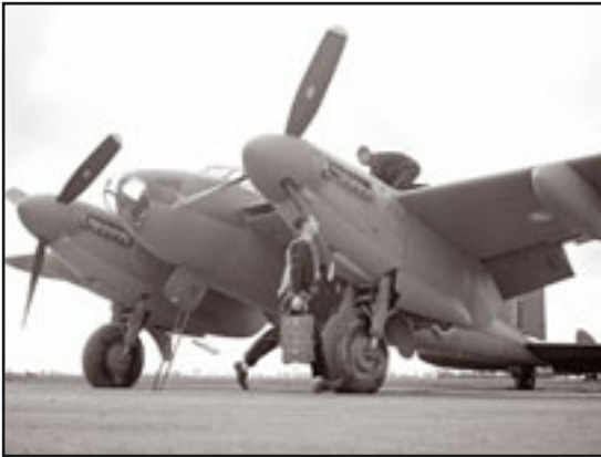
The Mosquito, one of the aircraft most tolerant of damage, was made of laminated plywood.
