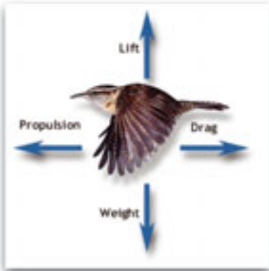
The illustration shows the main forces acting on a bird during flight.
